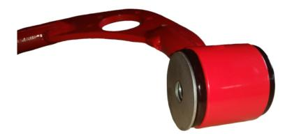
**The proper orientation:** Shear bolt head, 0.156" (thick) washer, black bushing, red bushing sleeve, black bushing, 0.074" (thin) washer, UCA tube mounted to the chassis, other side 0.074" (thin) washer, black bushing, red bushing sleeve, black bushing, 0.156" (thick) washer, and nut.
