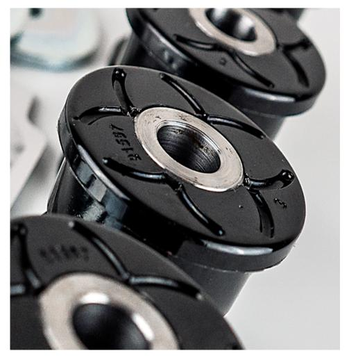
JBA has a patent on our control arm bushings. The EZ lube bushings have grease ports with a check valve. There is no need to loosen the mounting bolts to release the grease pressure.
